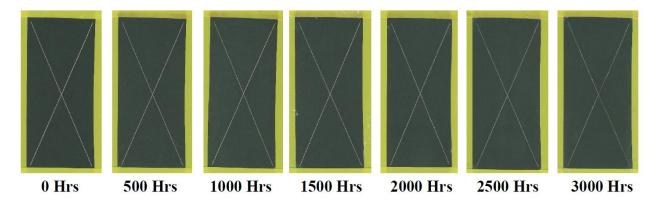
Figure 3. Corrosion Protection Of 2024-T3 Aluminum Alloy In ASTM B-117 Salt Fog Testing
